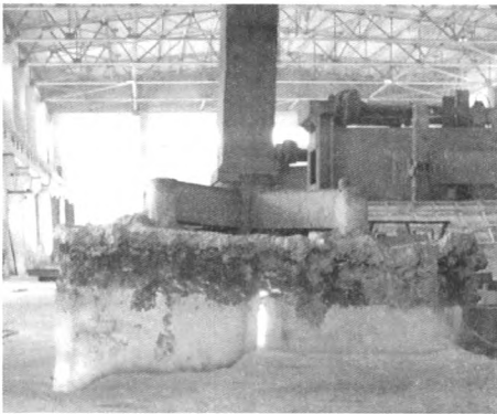
图 1 阳极角部伸腿肥大现象 Fig.1 The anode angle leg growth phenomenon
