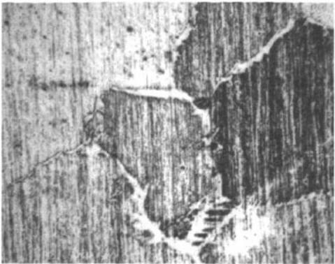
图 3 阀体基体显微组织形貌,400× Fig.3 Micro-structure of valve's substrate
