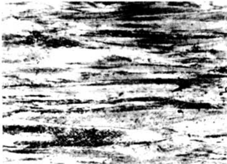
图6 冷加工变形组织,100× Fig. 6 Microstructure deformed by cold processing
