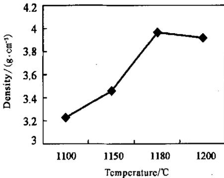
Fig. 4 Influence of sintering temperature and hours on volume
