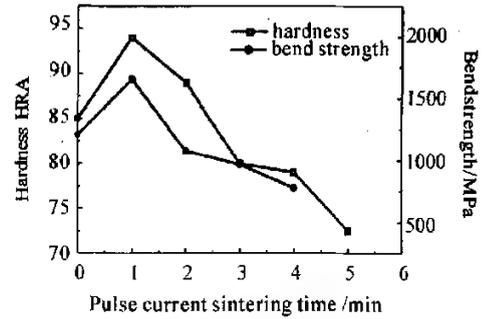
Fig. 4 Effect of pulse current sintering time on hardness and bend strength of sintered alloys (total sintering time 6min)
