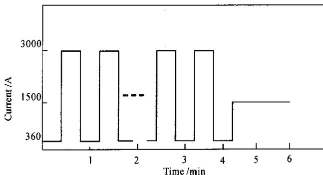
Fig. 2 Schematic diagram of current sintering process
