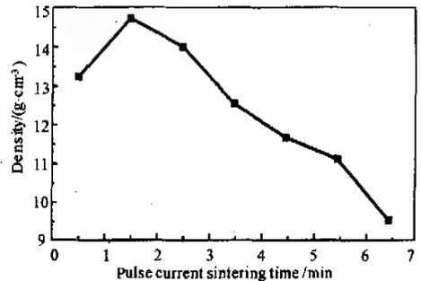
Fig. 3 Effect of pulse current on sintered density (total sintering time 6min)
