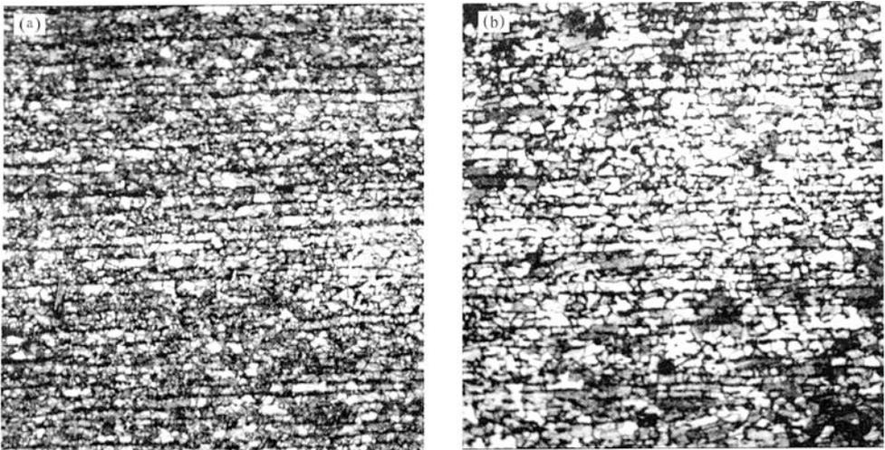
Fig. 1 Microstructure (X 100) of hot sheet from steel Cr3(GOST1577-81)
