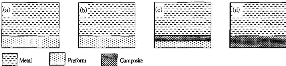
Fig. 2 A sketch showing the different infiltration cases in infiltration casting
