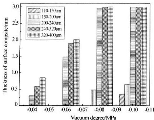
Fig. 5 Effect of grain size on the thickness of surface composite
