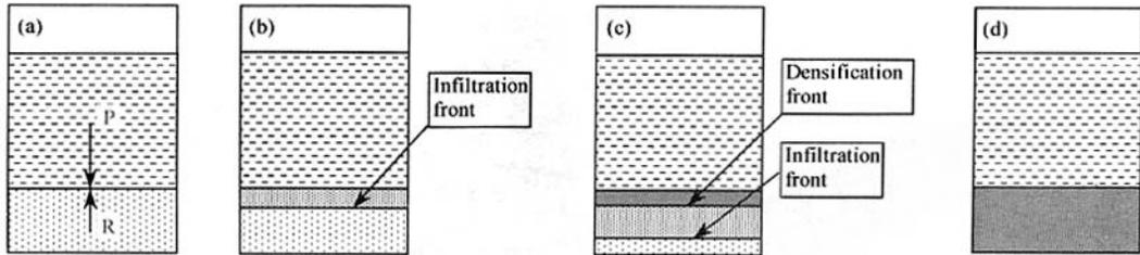
Fig. 7 A sketch of the infiltration in vacuum infiltration casting
