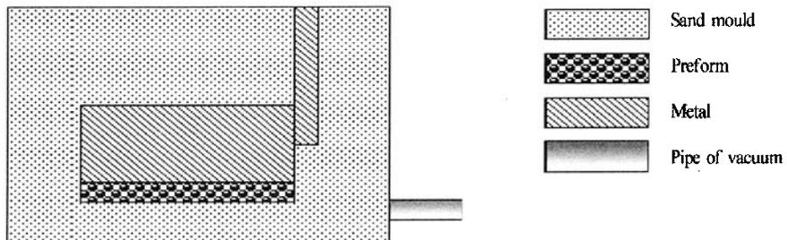
Fig. 1 Schematics of process to fabricate surface composite
