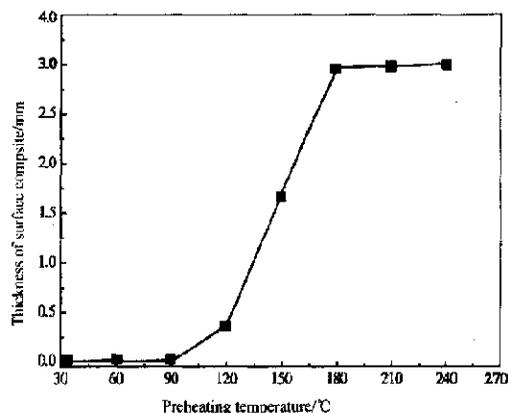
Fig. 6 Effect of preheating temperature on the thickness of surface composite
