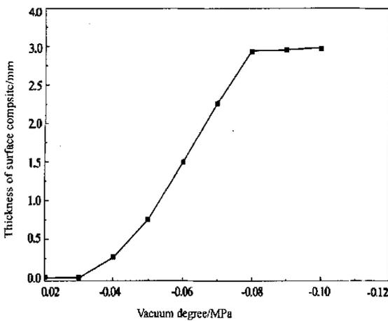
Fig. 3 Effect of vacuum degree on the thickness of surface composite
