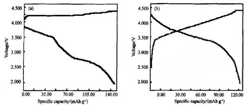
Fig. 2 Charge/discharge curves for the 1st cycle (a)-Sample A; (b)-Sample B
