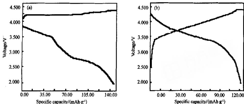
Fig. 2 Charge/discharge curves for the 1st cycle
