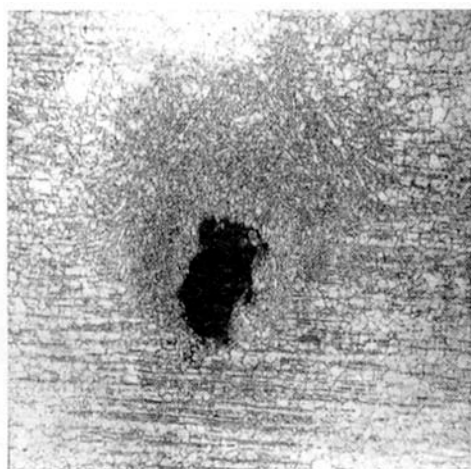
Fig. 2 Microstructure of the tiny holes in the \text{AgNi}_{10}/\text{CuNi}_{20} composite strip, 50 \times
