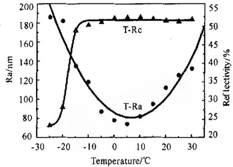
Fig. 2 Effect of electropolishing temperature on surface roughness and surface reflectivity
