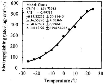
Fig. 1 Effect of electropolishing temperature on electropolishing rate
