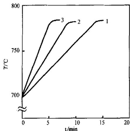
Fig. 2 Temperature-time diagrams in initial period of reduction at various sodium addition rates
