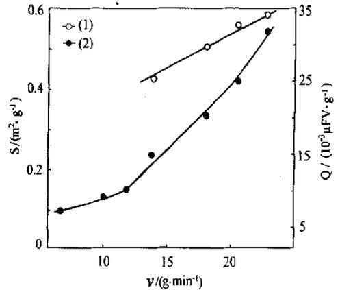
**Fig. 3** Dependencies specific surface (1) of powders and specific charge of anodes (2) on rate of sodium injection
