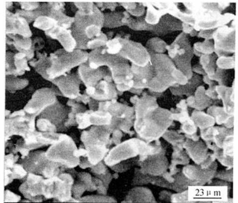
Fig.1 SEM photomicrograph of the Ti-based getter
