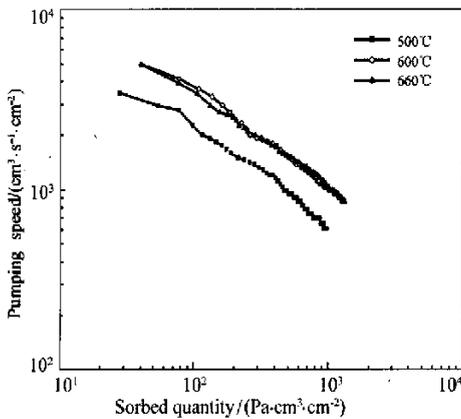
Fig.3 Gettering characteristic for H<sub>2</sub> at room temperature after activations at different temperatures
