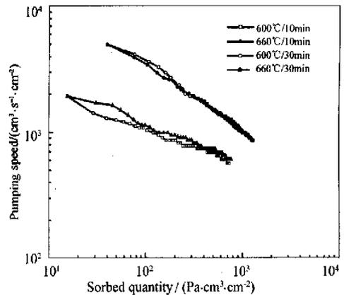
Fig.4 Comparison of gettering characteristic for H<sub>2</sub> at room temperature after different activation processes
