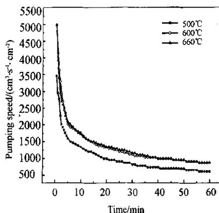
Fig. 2 Pumping speed for  $H_2$  at room temperature after activations at different temperatures
