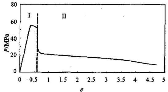
Fig. 2 The diagram of deformation of an alloy 30Cr8Co at complex loading at temperature 750 °C with a section of compression ( I ), torsion ( II )
