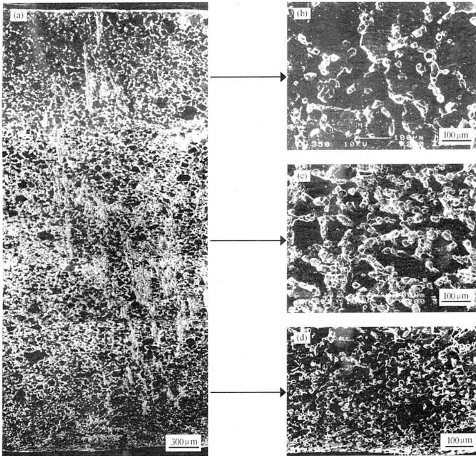
Fig. 3 A microstructure in a zone of active deformation of a sample of an alloy 30Cr8Co after deformation at temperature 750°C.
