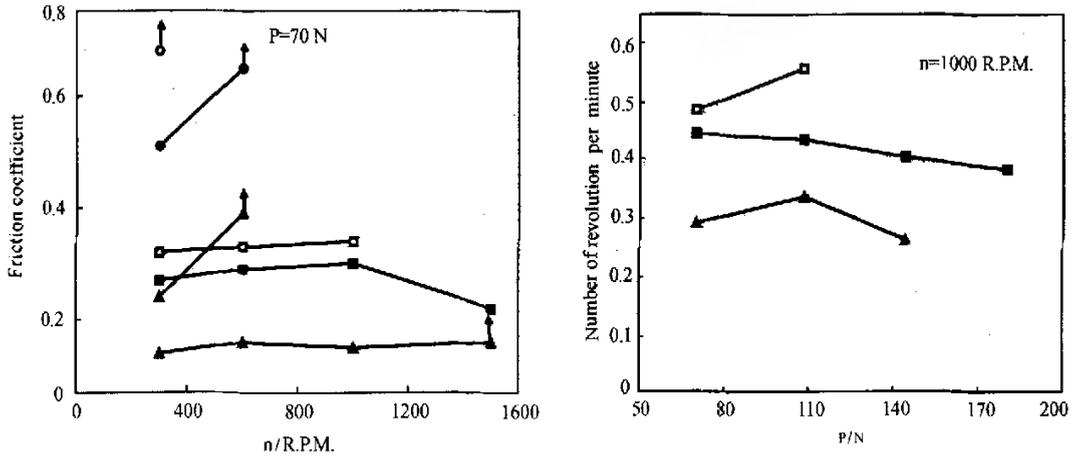
Fig. 3 Coefficient of friction of MMCs versus the sliding speed (a) and the applied load (b)
