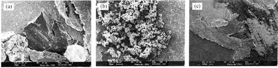
Fig.2 SEM micrographs of wear fragments collected at the end of the test at varied applied loads: plate-like flake (a), fine equiaxed particles (b) and a mixture of particles and flakes (c)
