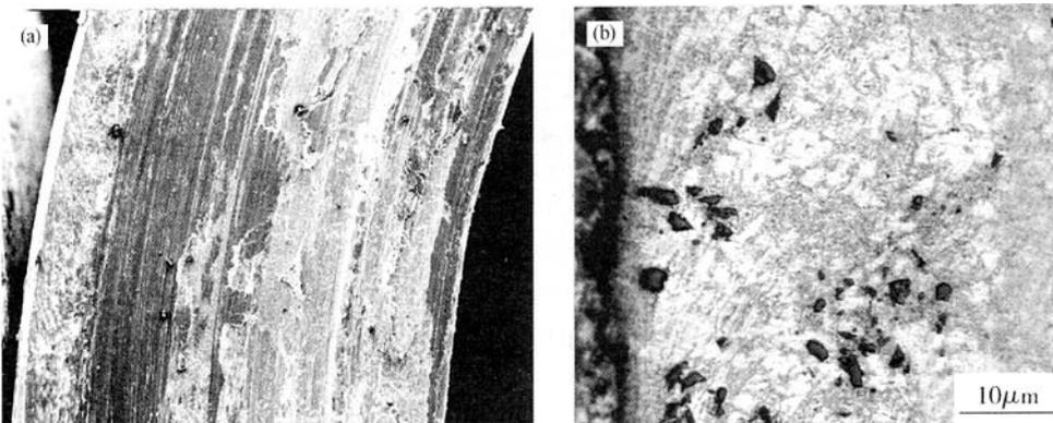
**Fig.1 SEM of worn surface (a) and optical micrographs of cross section of MMC after wear test (b)**
