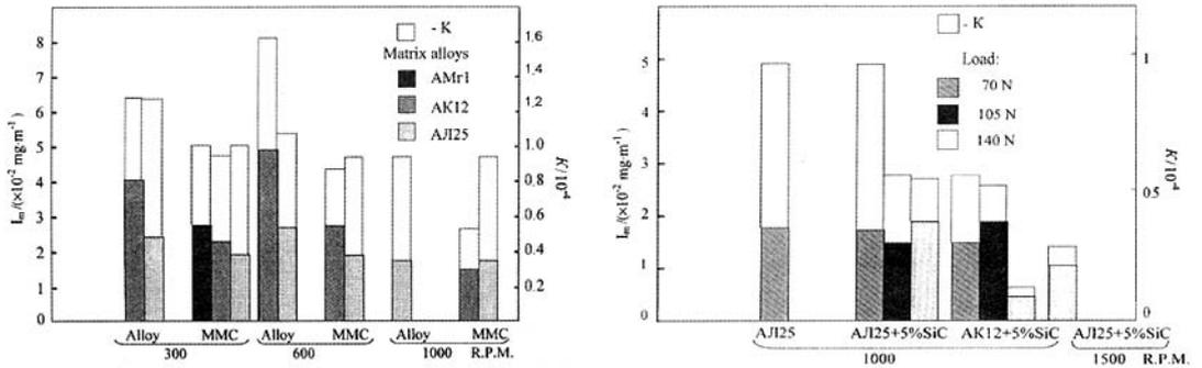
Fig.4 Sliding wear rates  $I_m$  and wear coefficients  $K$  of MMCs versus the sliding speed (a) and the applied load (b)
