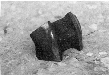
Fig. 4 The wear of friction slide block
