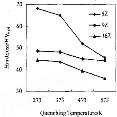
Fig. 5 Relationship between annealing temperature and the hardness of alloys
