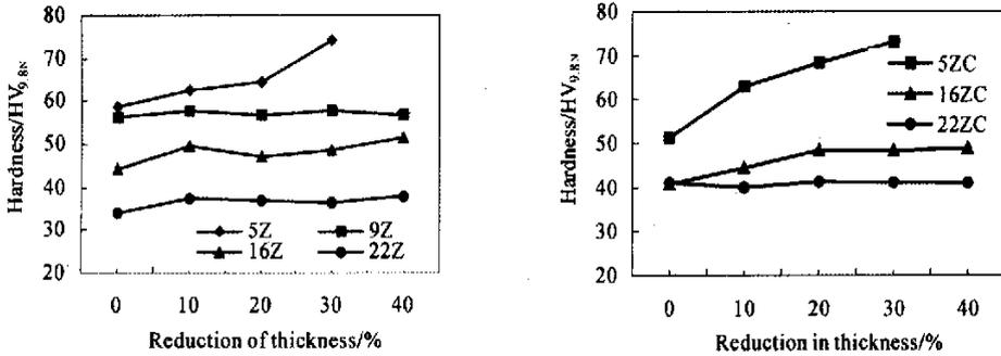
Fig. 4 Work-hardening curves for cold-rolling of Mg-Li-Zn and Mg-Li-Zn-2Ca alloys
