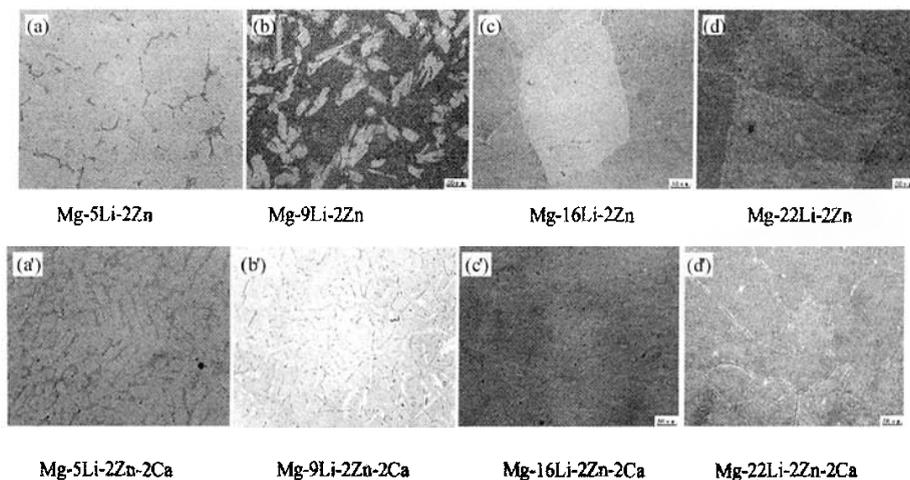
Fig. 1 Microstructure of as-cast alloys
