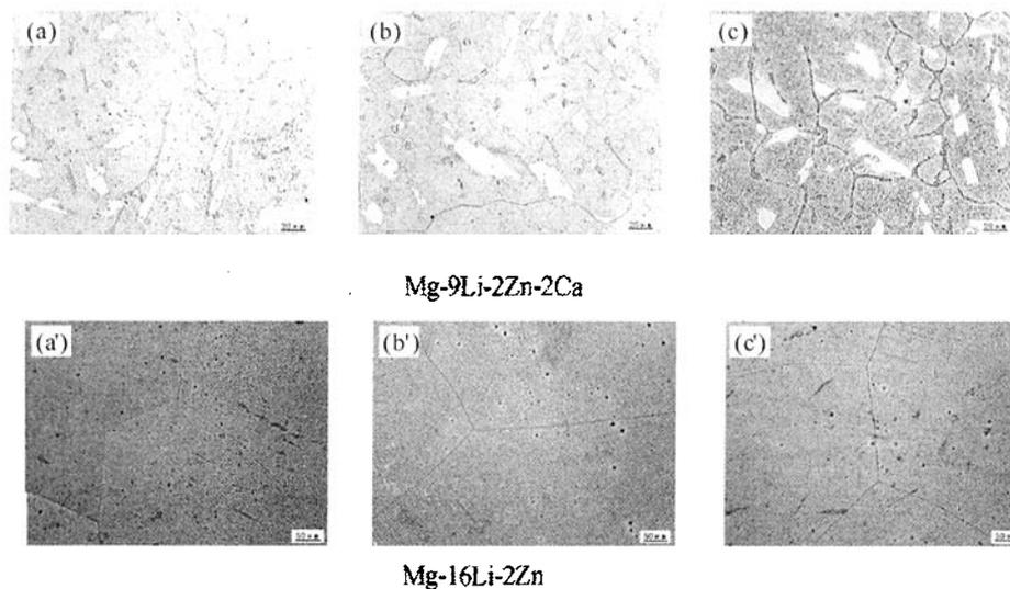
Fig. 2 Microstructure of different homogenized alloys
