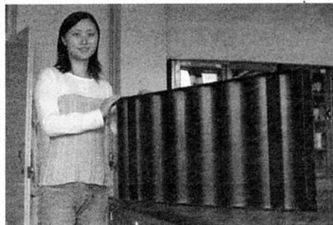
Fig. 13 Manufacturing system for RTM under development at LAC/BIAM and sine wave beam manufactured on this platform
