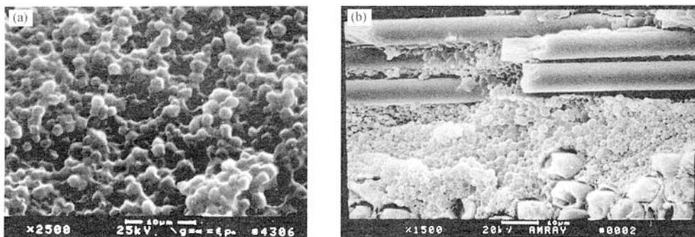
Fig. 1 (a) Phase-inversed granular morphology of resin cast resulting from spinodal decomposition (b) Interlaminar morphology of intercalated graphite laminate denoted as Case 1 in Table 1 indicating again the granular structure. In both cases, the TP continuous phase was chemically etched away
