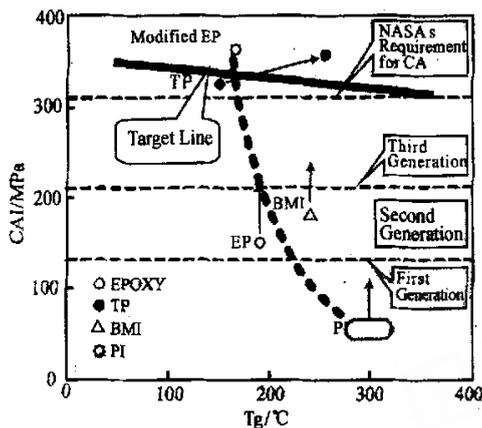
Fig. 12 Resin-dominant properties for graphite composites and the development target at LAC/BIAM
