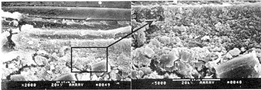
Fig. 6 Representatives<sup>[8]</sup> of interply morphology of BMI laminate toughened with PEK/BMI two-component film (60:40) by *ex-situ* concept
