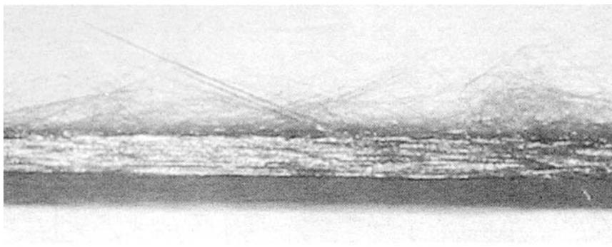
**Fig. 3** Representative of fiber pull-out after GIC testing
