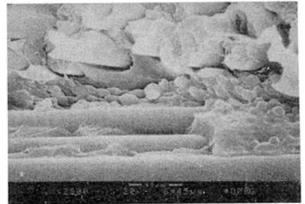
Fig. 11 Interlayer morphology of EP based graphite laminate manufactured by *ex-situ* RTM method<sup>[12]</sup>
