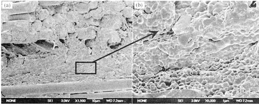
Fig. 7 (a) representative<sup>21</sup> of interlayer morphology of BMI laminate toughened with pure PEK film by *ex-situ* method; (b) A high magnification of (a)
