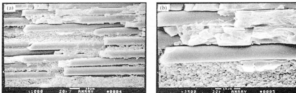
**Fig. 2** Boundary region between the two-phase granular and the pure EP structure within single graphite ply (a) and the high magnification of the sample in (b)
