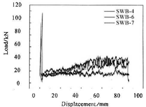
**Fig. 16** Mechanical response of different composite beams in crush test
