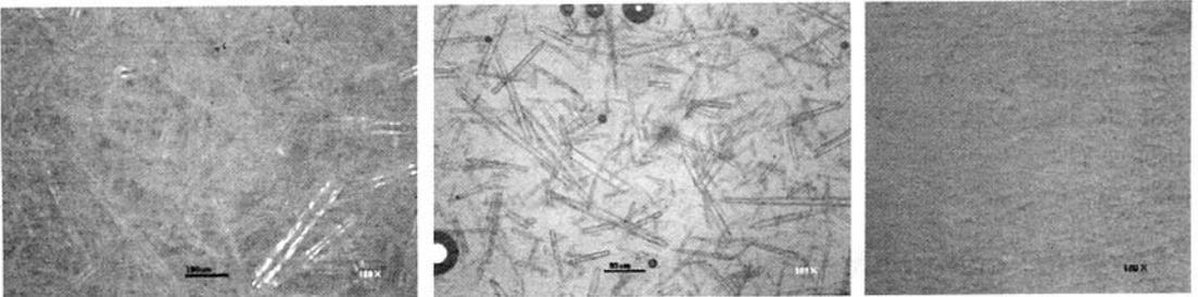
Fig. 9 Representatives<sup>[7]</sup> of phase change of a two-part BMI resin system at the beginning (a), in-between (b) and at the end (c)
