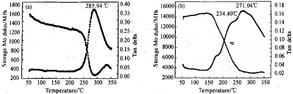
Fig. 5 Glass transition behavior of neat BMI (a) and the graphite laminate (b) made by *ex-situ* method
