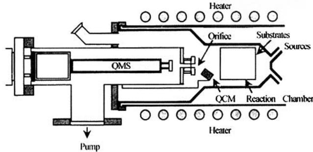
Fig. 2 Configuration of the ALD equipment
