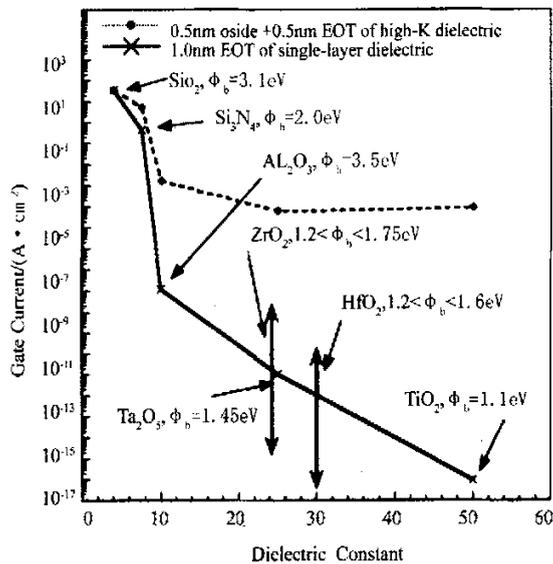
Fig. 3 Tunneling currents through different dielectrics
