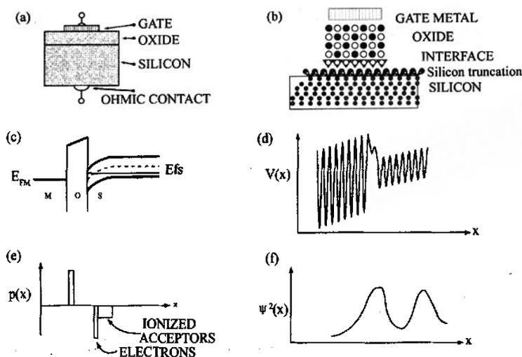
Fig. 1 Comparison between the classical view and the atomic-layer view of a MOS capacitor
