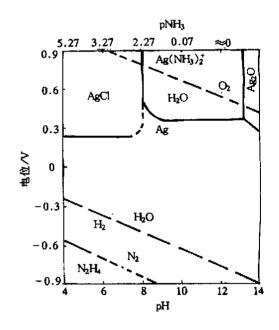
图 2 AgCl-NH<sub>3</sub>-H<sub>2</sub>O 系电位-pH 图  $[Ag(NH_3)_{2}^{+}] = 0.5 \text{ mol/L}, [Cl^{-}] = 0.6 \text{ mol/L}, \\ [NH_3]_{7} = 1 \text{ mol/L}, p(O_2) = p(H_2) = 1 \times 10^5 \text{ Pa}$ Fig. 2 E<sub>H</sub>-pH diagram for AgCl-NH<sub>3</sub>-H<sub>2</sub>O
