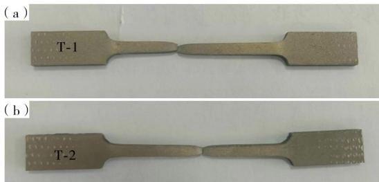
(a)—母材;(b)—搅拌摩擦焊件。 (a)—the base metal;(b)—the friction stir welding parts.
